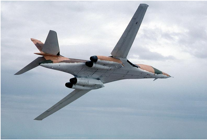
Figure 23. B-1A, with wings fully extended for low-altitude flight; compare with Fig. 24.
