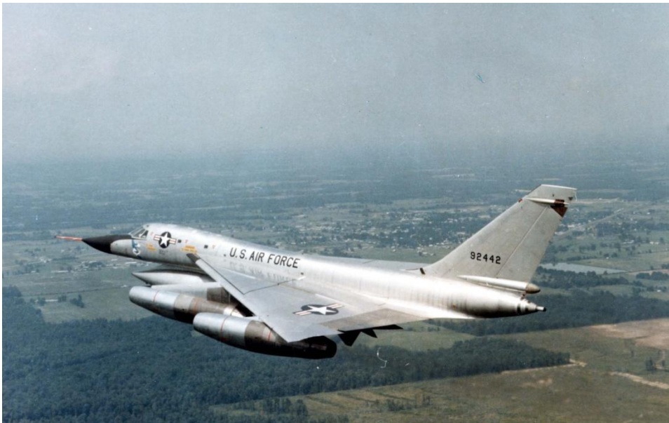
Figure 19. This photograph of a B-58 was taken in June 1967. Note the tail-less delta wing design and fuel pod under the fuselage.
