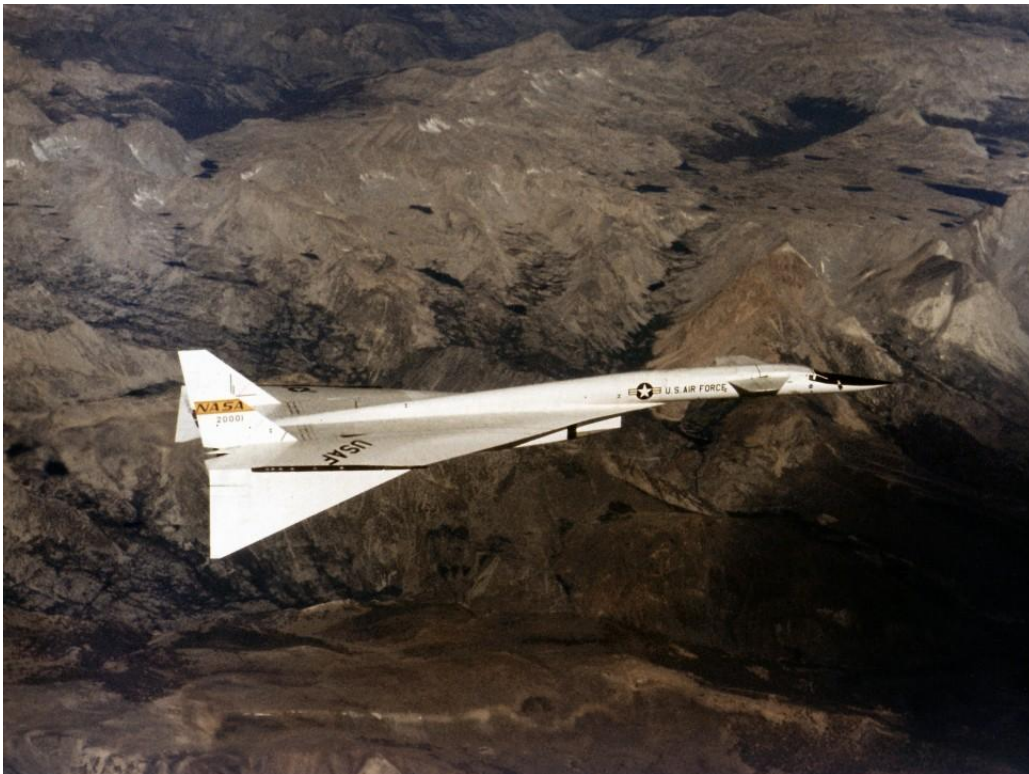
Figure 21. A B-70 prototype on a test flight in the 1960s. Note the wing tips in the down position.
