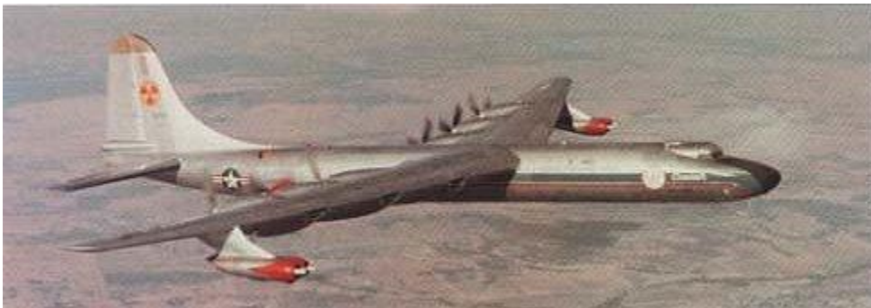
Figure 15. The NB-36, test bed for a potential nuclear-powered U.S. bomber. A similar Soviet program may have advanced beyond the preliminary testing stage of its U.S. counterpart.
