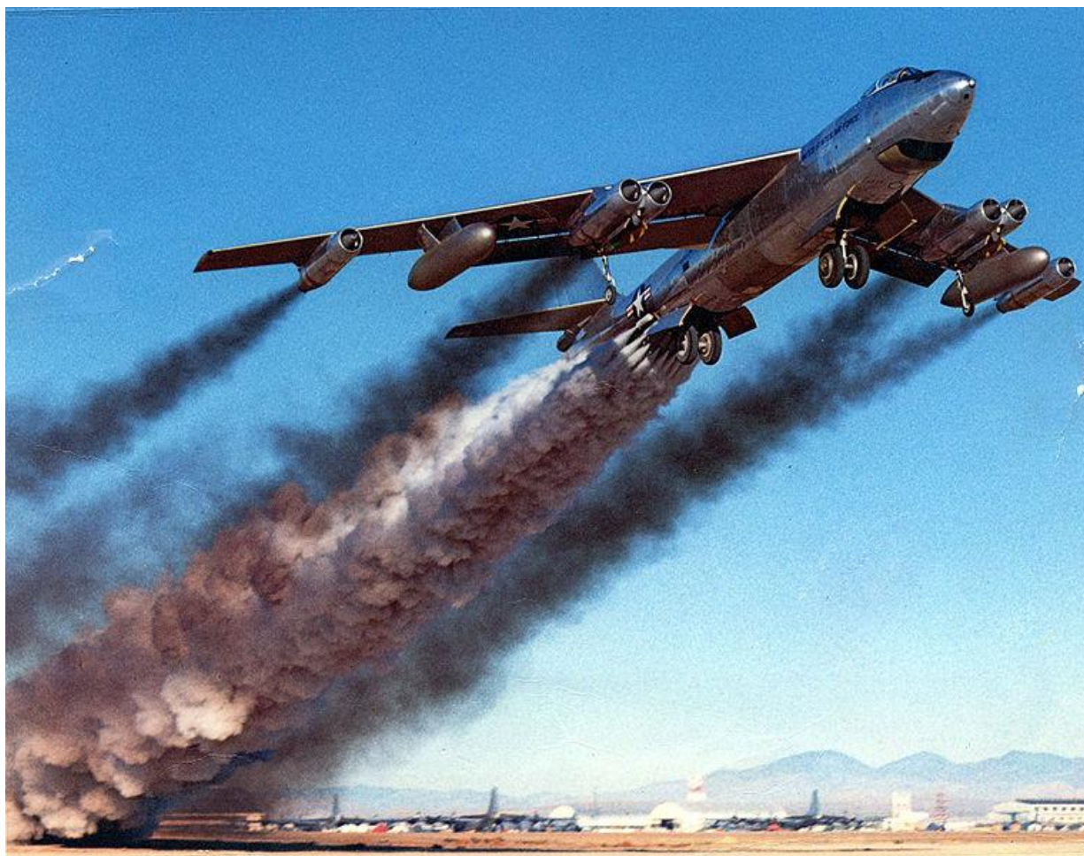
Figure 16. A B-47 on takeoff. Note the tan smoke from the RATO rockets and the innovative “bicycle” undercarriage with outriggers on the wings. The pods roughly \frac{2}{3} outboard on each wing are merely auxiliary fuel tanks.
