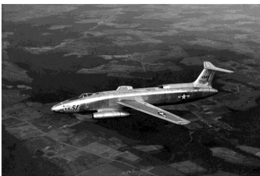
Figure 10. Martin XB-51. Note the highly swept wings, high T tail, and three engines.
