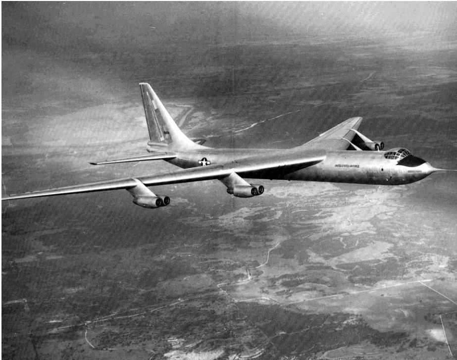
Figure 18. The YB-60, probably in mid 1952. It was clearly a derivative of the obsolete B-36, and it was passed over in favor of the similar B-52.
